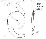
**Lens Type** Single Piece, Aspheric Optic, 360° Square Edge
